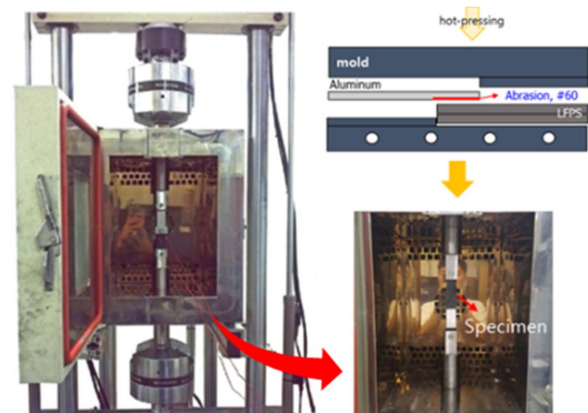
Fig. 6. Environmental test setup for temperature condition
