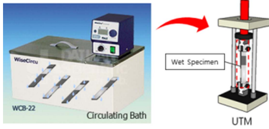
Fig. 7. Environmental test setup for moisture exposure
