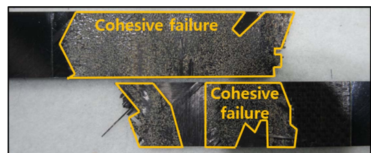
Fig. 10. Typical failure mode (0 atm, heat-blanket)
