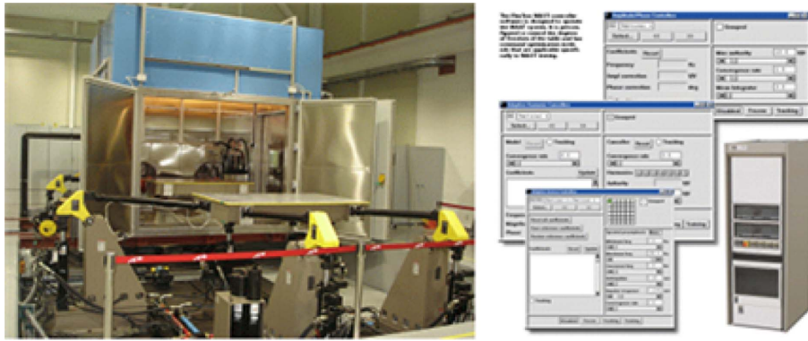
Fig. 7. Photograph of MAST(MTS model 323.40)
