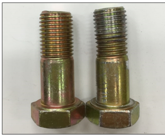
(a) Bolts before (left) and after (right) test
