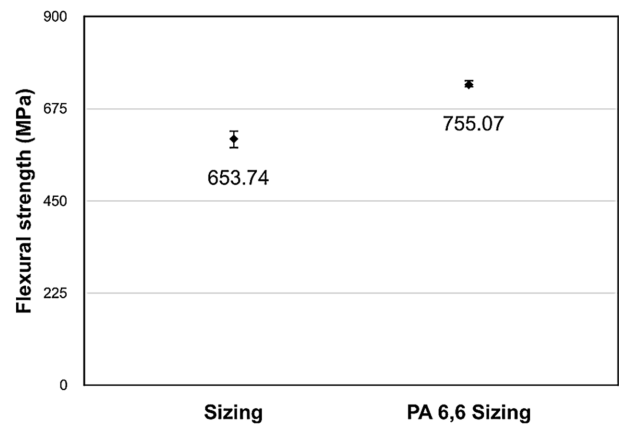
Fig. 9. Flexural strength results of CFRTs with respect to sizing method
