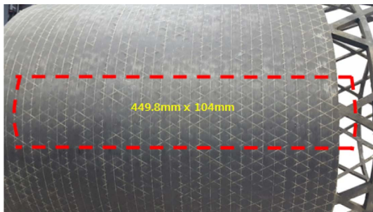
Fig. 2. Composite lattice structure (rib structure with skin)
