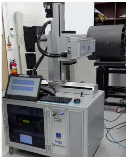
Fig. 3. Inspection of composite lattice structure using pulse echo ultrasonic propagation imaging system
