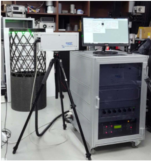
Fig. 15. Inspection of composite lattice structure using guided wave ultrasonic propagation imaging system
