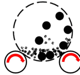
Fig. 1. Schematic representations of ball-mill process
