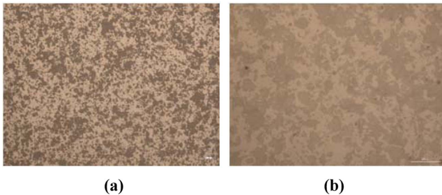
Fig. 3. Optical micrograph of EBC surface after coating process at spray distance of 100 mm with different magnification (a) x50 and (b) x200
