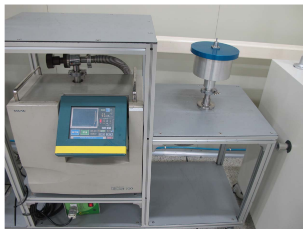
Fig. 5. Leak detector used for testing seal performance. The ferrofluid seal was positioned at the upper part of chamber
