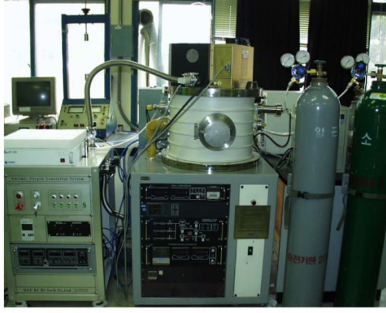
(a) Picture of the accelerated LEO simulation facility
