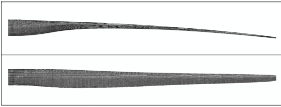
Fig. 3. FE mesh model for structural analysis
