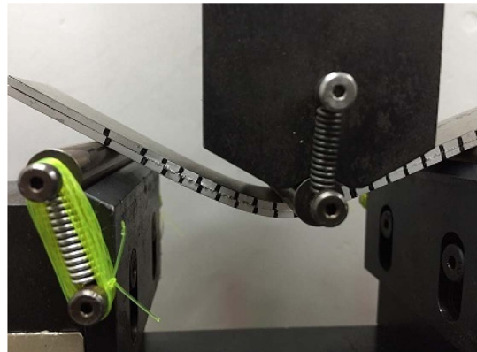
Fig. 6. Fracture during ENF test
