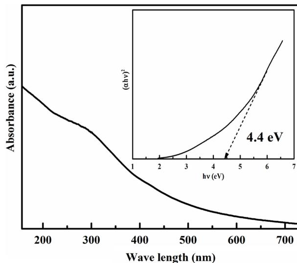
Fig. 5. UV-vis. absorption spectra of NiO/Fe<sub>3</sub>O<sub>4</sub>. The inset view shows the corresponding  $(ah\nu)^2$  vs.  $h\nu$  plot
