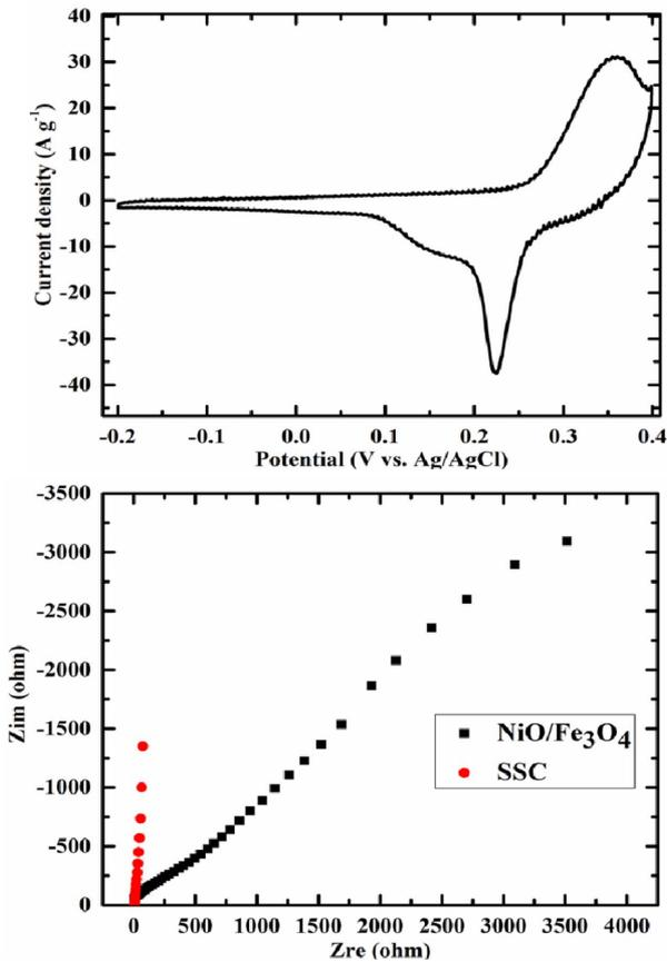
**Fig. 6.** (a) CV of NiO/Fe<sub>3</sub>O<sub>4</sub> (b) Nyquist plot of NiO/Fe<sub>3</sub>O<sub>4</sub> and SSC device
