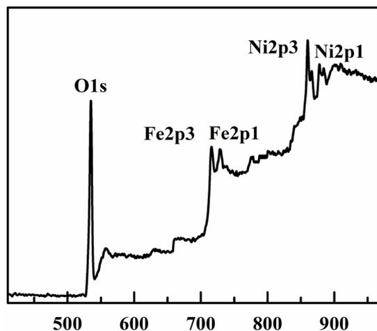
Fig. 3. XPS survey spectra of NiO/Fe<sub>3</sub>O<sub>4</sub>
