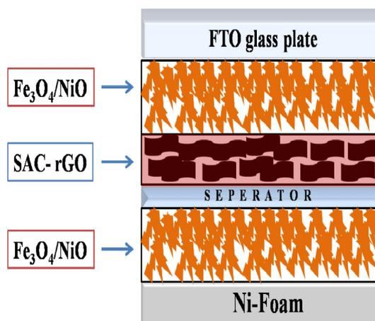
Fig. 2. Schematic representation of two electrode SSC device
