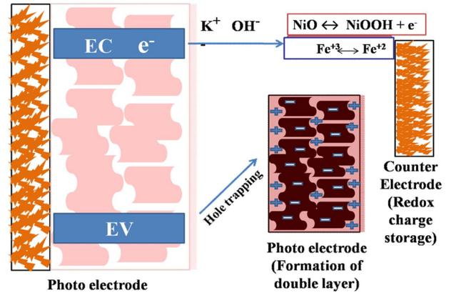
**Fig. 7.** Schematic representation of the charging mechanism of SSC device
