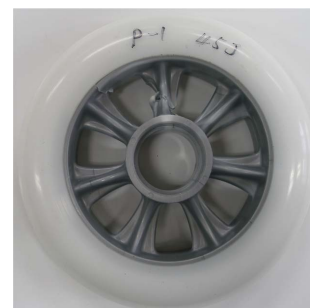
Fig. 11. Fracture of plastic wheel (45 J impact)
