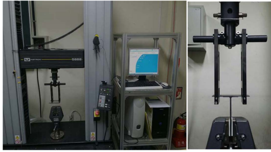
Fig. 3. Static tensile test set-up
