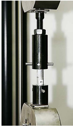
Fig. 9. Butt test for observation of traction stress
