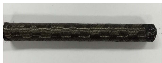
Fig. 1. SiC fiber preforms of SA3-S1I08PX helically wound with winding angle of +55/-55^\circ on the Zircaloy-4
