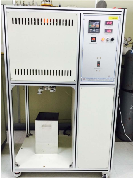
Fig. 6. drop tube furnace for thermal shock test
