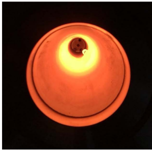
Fig. 7. Interior of furnace where specimen was installed (1200°C)
