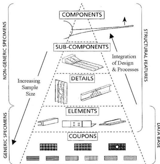
Fig. 6. Schematic diagram of building block tests for a fixed wing [26]
