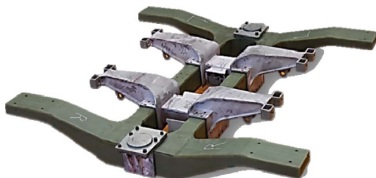
Fig. 1. Bogie structure manufactured by autoclave molding process
