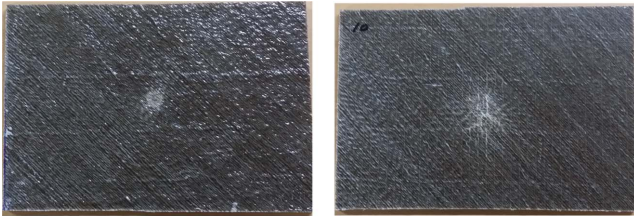
Fig. 10. Damage configuration of specimen after impact test (10 J)
