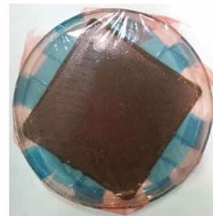
Fig. 4. Prepare for electrolyte coating
