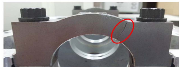
Fig. 13. Location of Fatigue Fracture
