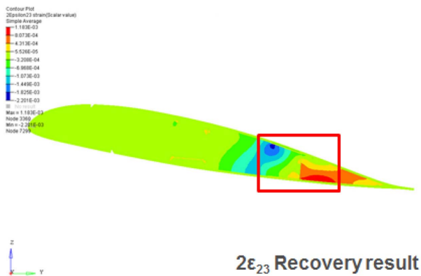
Fig. 9. 2\epsilon_{23} strain recovery analysis result for composite rotor blade
